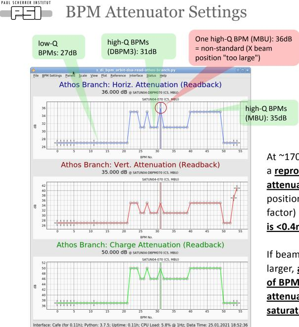
At ~170pC, each BPM type has a <u>reproducible standard RFFE</u> <u>attenuator</u> setting (and thus position and charge scaling factor) <u>as long as beam offset</u> <u>is <0.4mm</u>.
