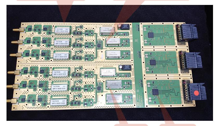
3-Channel RF front-end, 2<sup>nd</sup> cavity BPM 2-channel 16-bit 500MSPS ADC (JESD204B)
