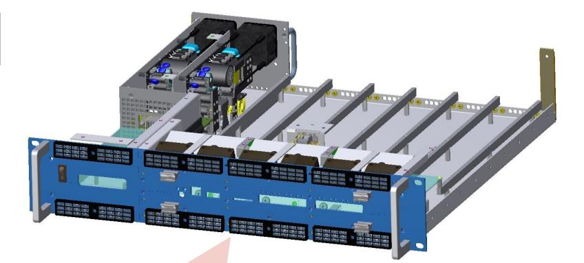
Air flow/ventilation optimized for high temperature stability & low BPM drift (suboptimal in VME-based solutions).
