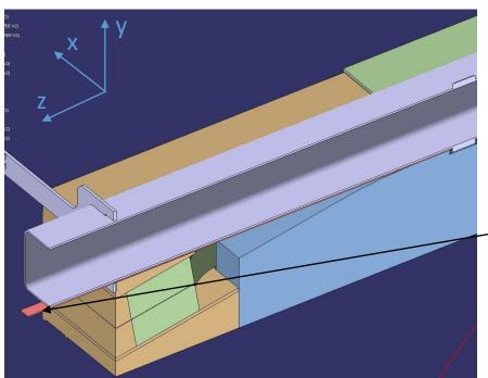
Removable shim for guaranteeing the "Y" position of the test well
