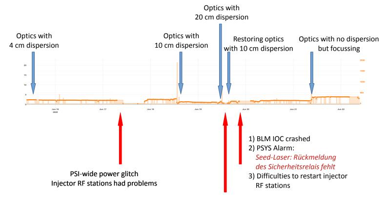
Dark current (!) losses in undulator after Fbs have been enabled
