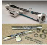
QMIR crab cavity by Fermilab/ANL: Up to 2 MV per cavity (0.5 m) Few HOMs, simpler cryomodule, Large impedance (smaller V-aperture).
