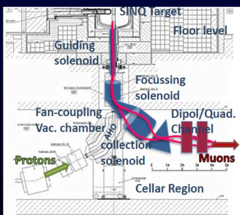
Fig. 4: HiMB concept showing extraction from the SINQ target (top) to the cellar region.
