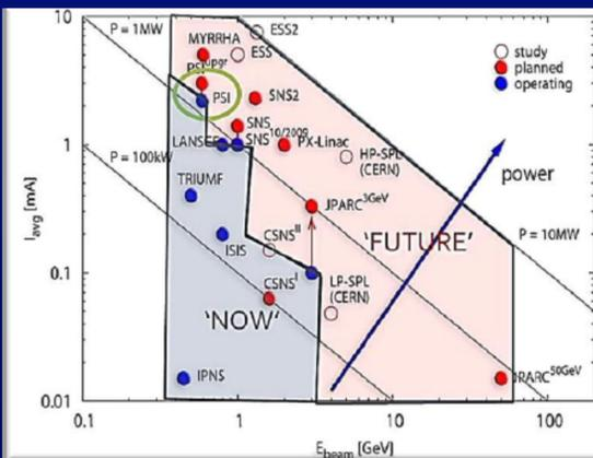
Fig. 1: The Intensity Frontier- current & future accelerator facilities around the world. The diagonal lines represent beam power contours of 0.1, 1 & 10 MW.
