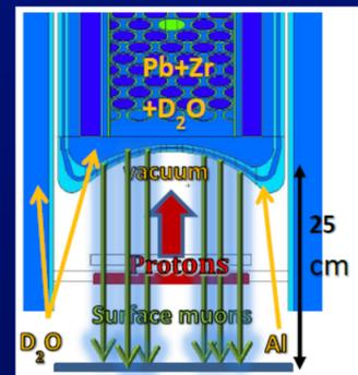
Fig. 5: PSI MCNPX Monte-Carlo model of SINQ Target region
