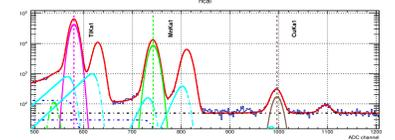
SDD spectrum recorded with a  $^{55}\text{Fe}$  source and a Ti foil at LNGS. Ti and Mn  $K\alpha$  lines are used for calibrating the energy spectrum. Residuals compared to the fit are also shown.
