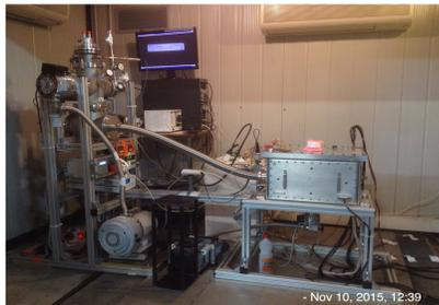
The vacuum chamber of VIP 2 at LNGS (right), which contains the Cu target and the detectors. The cryogenics needed to cool the SDDs is also visible (left).
