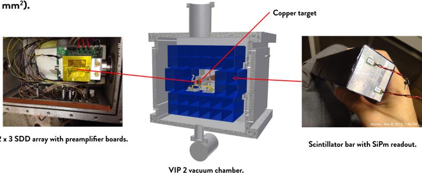
2 x 3 SDD array with preamplifier boards.
