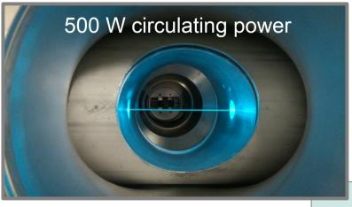
At 0.4 MW/cm<sup>2</sup> (0.7 kW circulating power) mirror degradation observed.
