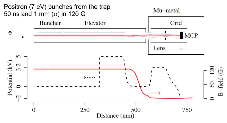
On target (kept at ground): positron bunches of 1 ns with a beam spot of 1 mm extracted to the field free e-m region with 90 % efficiency.
