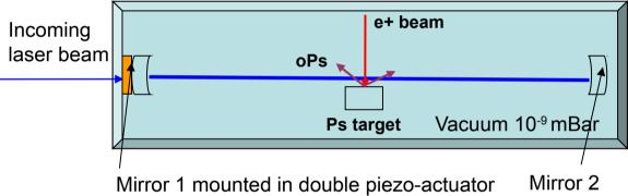
High finesse resonator for power build up 500 mW 1 kW
