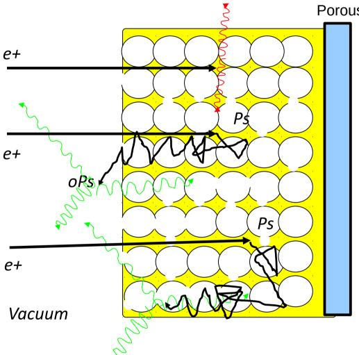
Porous Silica thin film ~1000nm 3-4 nm pore size
