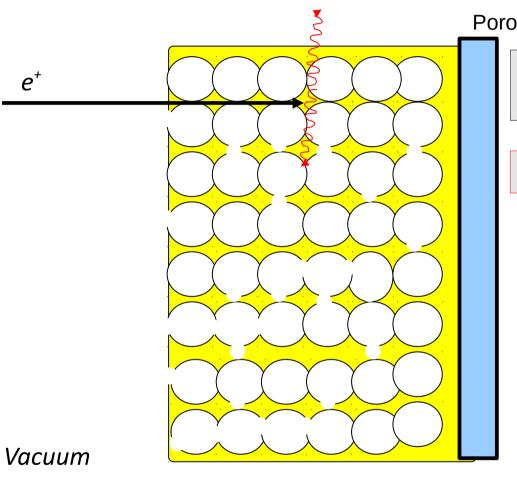
Porous Silica thin film ~1000nm 3-4 nm pore size
