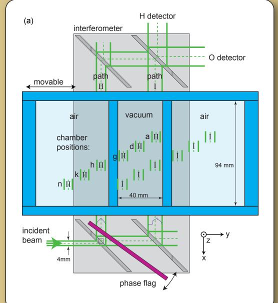
At the neutron interferometry setup S18 at the Institut Laue-Langevin (ILL) in Grenoble, monochromated thermal neutrons with a wavelength of 2.72Å and a FWHM of 0.043Å enter a perfect crystal silicon interferometer operated at a Bragg angle of 45°.
