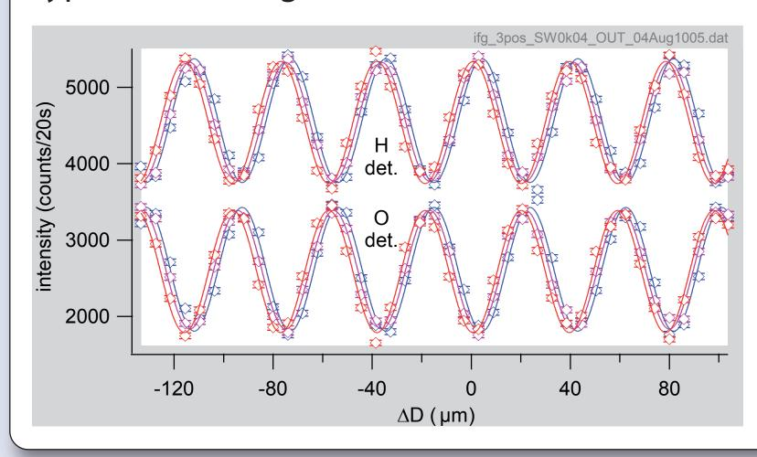
Recorded intensity oscillations between O- and H-detector as a function of the optical path length difference.
