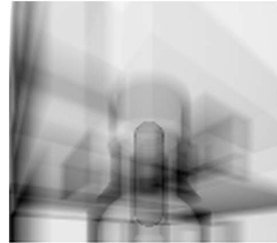
Transmission tomography scan of unit 1 indicates complete reactor meltdown (March 2015)
