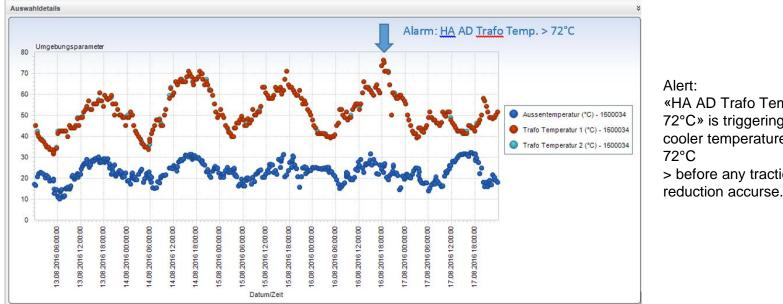
«HA AD Trafo Temp. > 72°C» is triggering when cooler temperature reaches > before any traction
